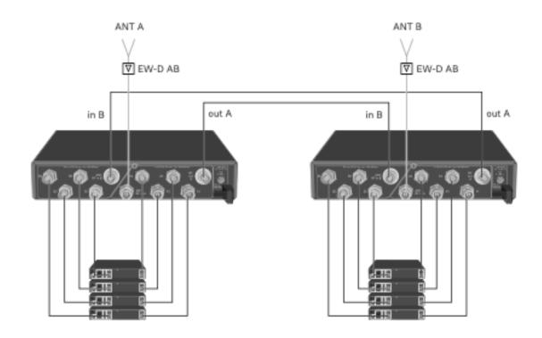
Option 3: Two antennas supply a 8-channel system
